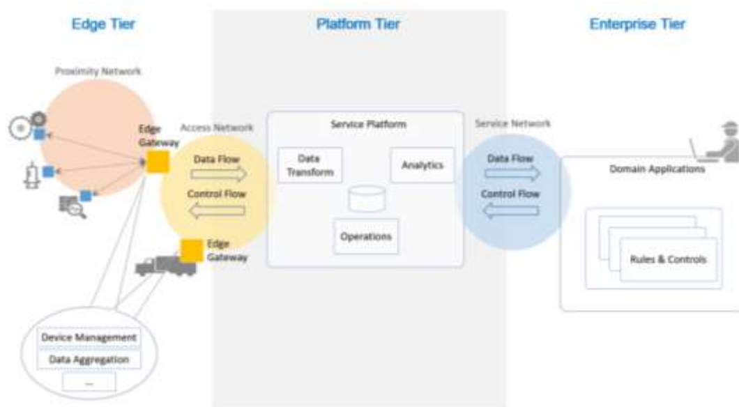
Figure 9 - Three-tier industrial IoT system architecture (Source: IIC [11])
